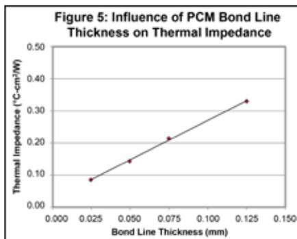
**Figure 5:** Influence of PCM bond line thickness on thermal impedance.
