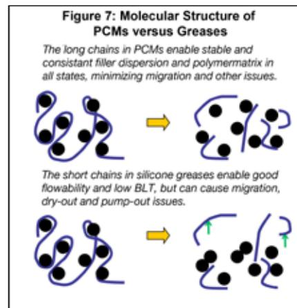
**Figure 7:** Molecular structure of PCMs vs. greases.
