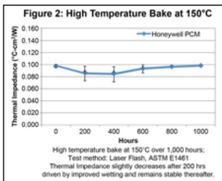
**Figure 2:** High-temperature bake performance of PCMs.
