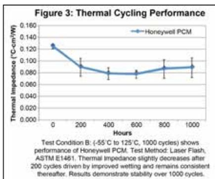
**Figure 3:** Thermal cycling performance of PCMs.
