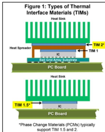
Figure 1: Types of thermal interface materials (TIMs).
