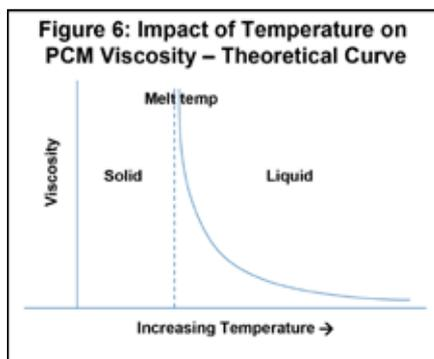
**Figure 6:** Impact of temperature on PCM viscosity.
